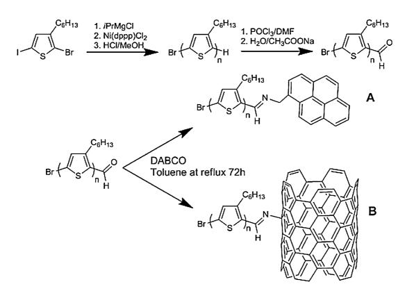
Scheme 1. Synthetic route to functional P3HT for physisorption (A) or chemical grafting (B) on nanotubes.
