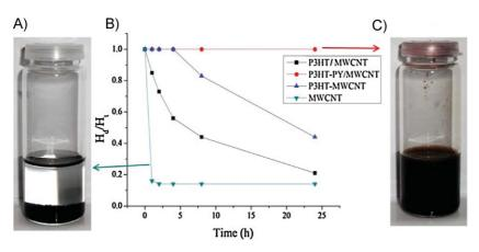
*Figure 1.* (A) Photograph of MWCNTs in THF after 2 h (B) Result of the sedimentation test for the three studied materials and pristine MWCNTs (C) Photograph of MWCNTs in a P3HT-Py solution in THF after 24 h.
