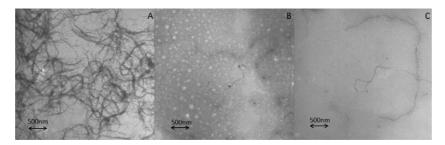
Figure 2. TEM images of P3HT/MWCNT (A); P3HT-Py/MWCNT (B); P3HT-MWCNT (C) prepared from 0.25 mg  $\cdot$  mL<sup>-1</sup> chlorobenzene solutions with 1 wt.-% of MWCNTs.
