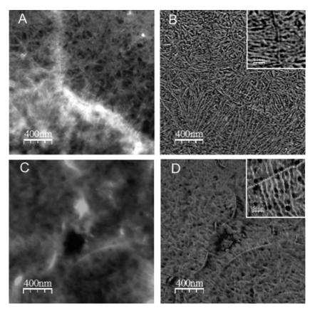
*Figure 3.* Tapping-mode AFM height (A) vertical scale 45 nm, C-vertical scale 70 nm) and phase (B,D) images of thin deposits of P3HT-Py/MWCNT 1 wt.-% (A,B) and P3HT-MWCNT 1 wt.-% (C,D). The insets in images B and D (scale bars: 80 and 56 nm, respectively) show close-ups on a single nanotube with P3HT fibrils arranged perpendicular to it.
